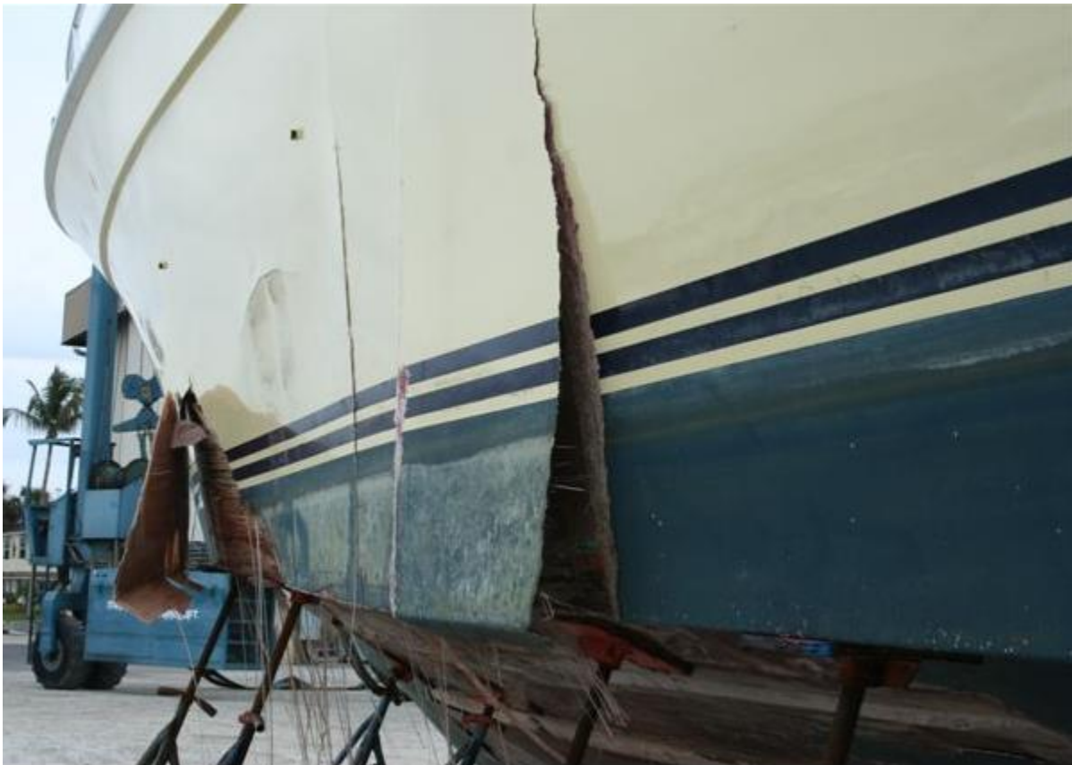
Photo of delamination between the outer skin and the core on a Bertram 63' Cruiser
